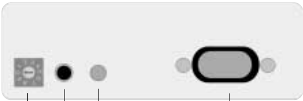
Channel selection switch Connection socket for vibrating pad On/off switch for acoustic signal Mains connection
