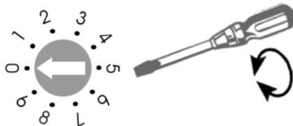
It is only necessary to set units to other channels if you have several different users operating units in the same building. Set the required channel by using a small screwdriver to turn the channel selector switch, which is located towards the top of the battery compartment, to the required channel number. All transmitters and receivers must be set to the same channel.
